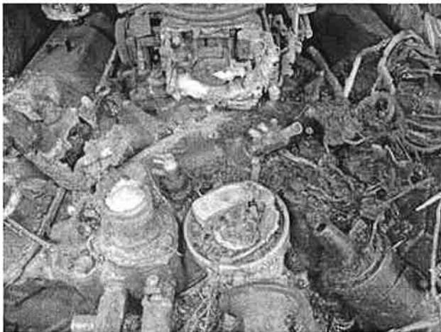
Pictures taken of engine after fire
