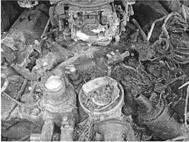
Pictures taken of engine after fire
