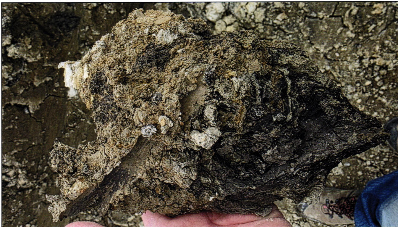
Figure 2: Close up photograph of uncontrolled fill soils observed during our site visit on June 26, 2026.
